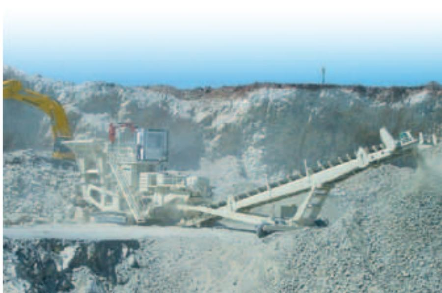
A mobile quarry application in Spain with a primary crushing plant LT140 and a TRLP12-20 conveyor.
