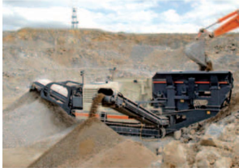
Fine materials can be removed before the crushing using a side conveyor.
