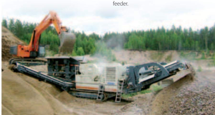
Road base materials crushed with LT3054 of natural gravel.
