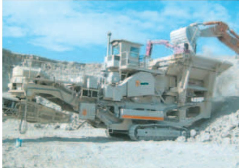
Mobile primary crushing for cement plant in the USA using LT140 + LL12.
