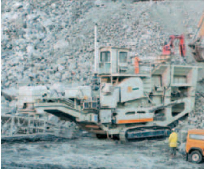
A quarry operation in the UK with Lokotrack LT140 and an LL12 mobile conveyor system.
