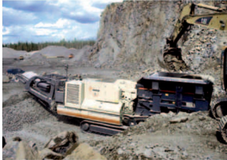
LT3054 features the one-button process start-up provided with the IC600 intelligent control system.
