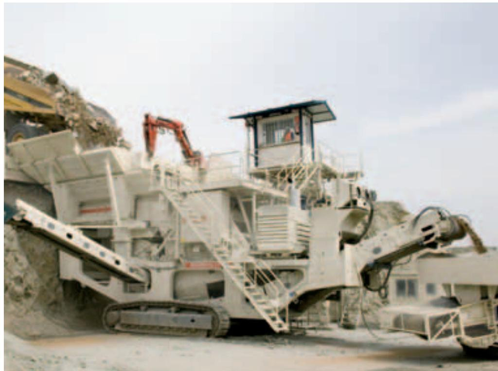
Lokotrack LT125 with an optional air conditioned control cabin.
