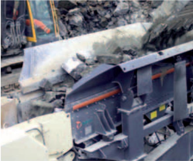
LT110 can be equipped with a high-capacity grizzly, a pan feeder/scalper or a roller grizzly.
