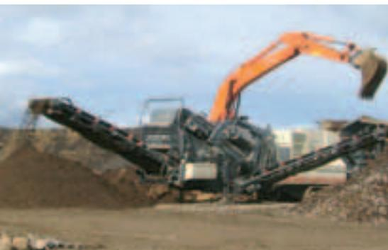
Lokotrack LT3054S, equipped with a screen module.
