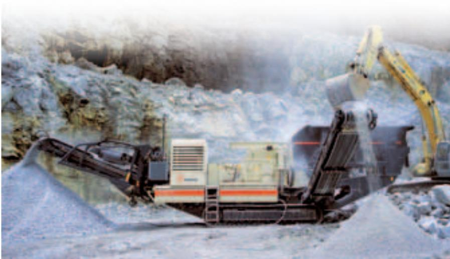
Crushing at a limestone quarry with Lokotrack LT1315.
