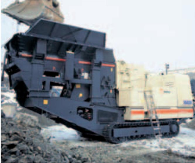
The large, 8 cubic metre feed hopper enables easy, continuous feeding.
