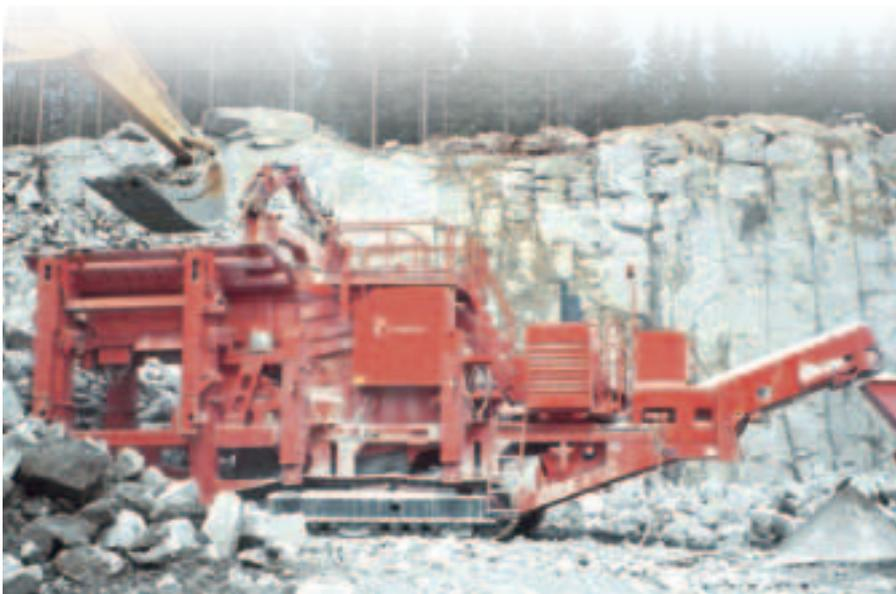
The "Split" model of Lokotrack LT125 is equipped with hydraulic legs for fast dismantling.
