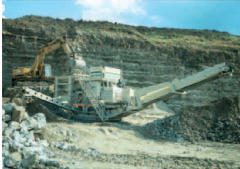
Primary crushing in the UK with Lokotrack LT125.
