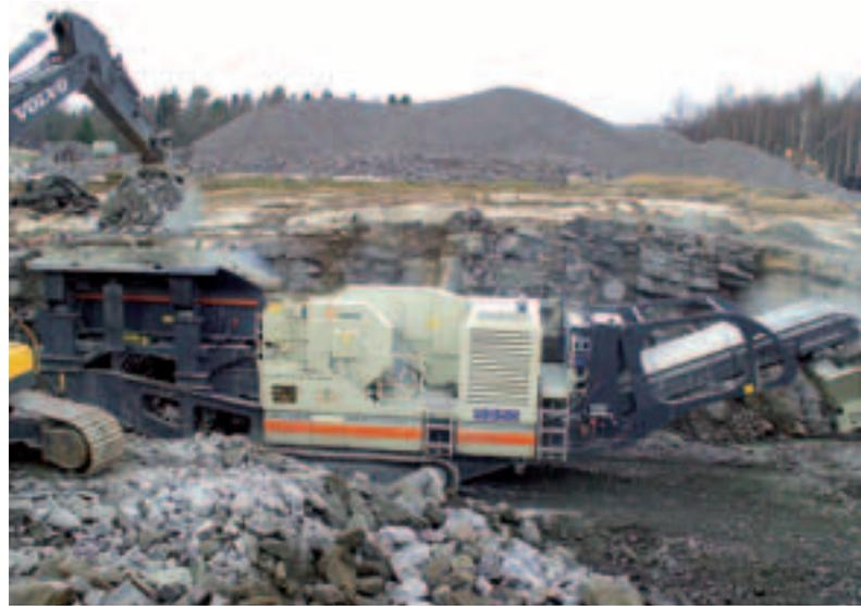
Primary crushing with Lokotrack LT110 in Sweden.
