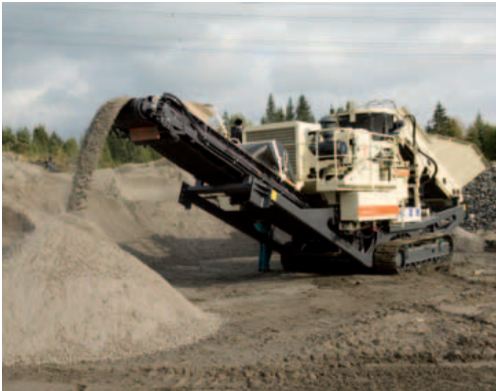
The new LT7150 allows the production of high quality cubical aggregates, and manufactured sand.
