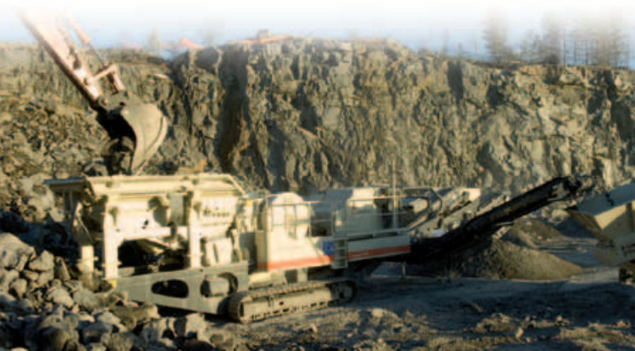
The screening unit can be disconnected in minutes allowing the Lokotrack LT106S to be used as a normal primary crushing unit.
