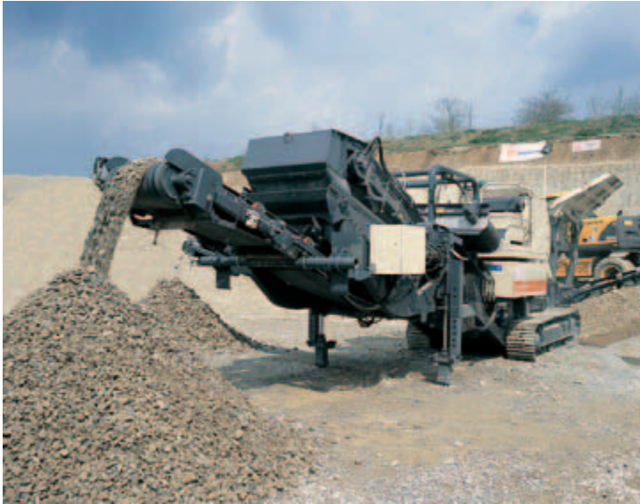
The detachable screen of the Lokotrack LT96S guarantees efficient classifying of the crushed materials into clean end products.
