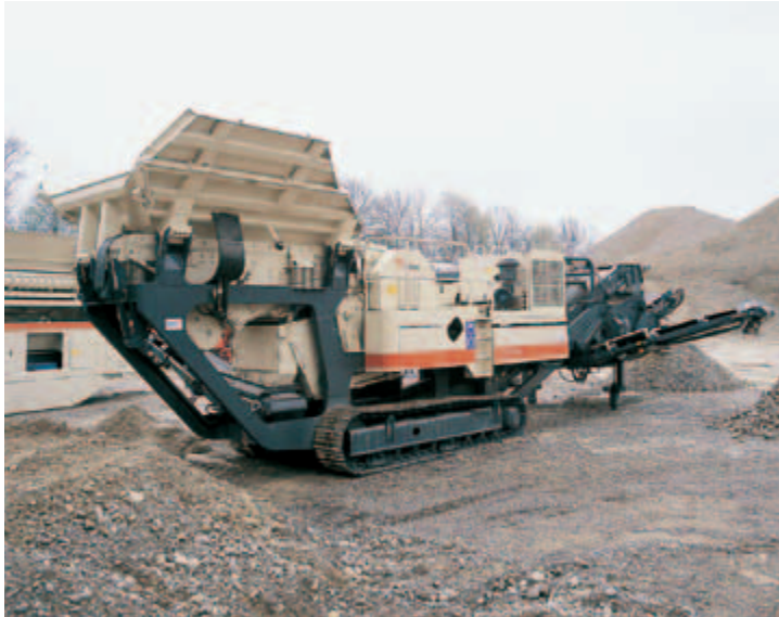
Sturdy, 4m³ or 6m³ Hardox steel feed hoppers can be chosen for the Lokotrack LT96S.
