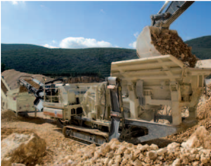
The sturdy feed hopper in LT1213 is manufactured from high-quality wear resistant steel.
