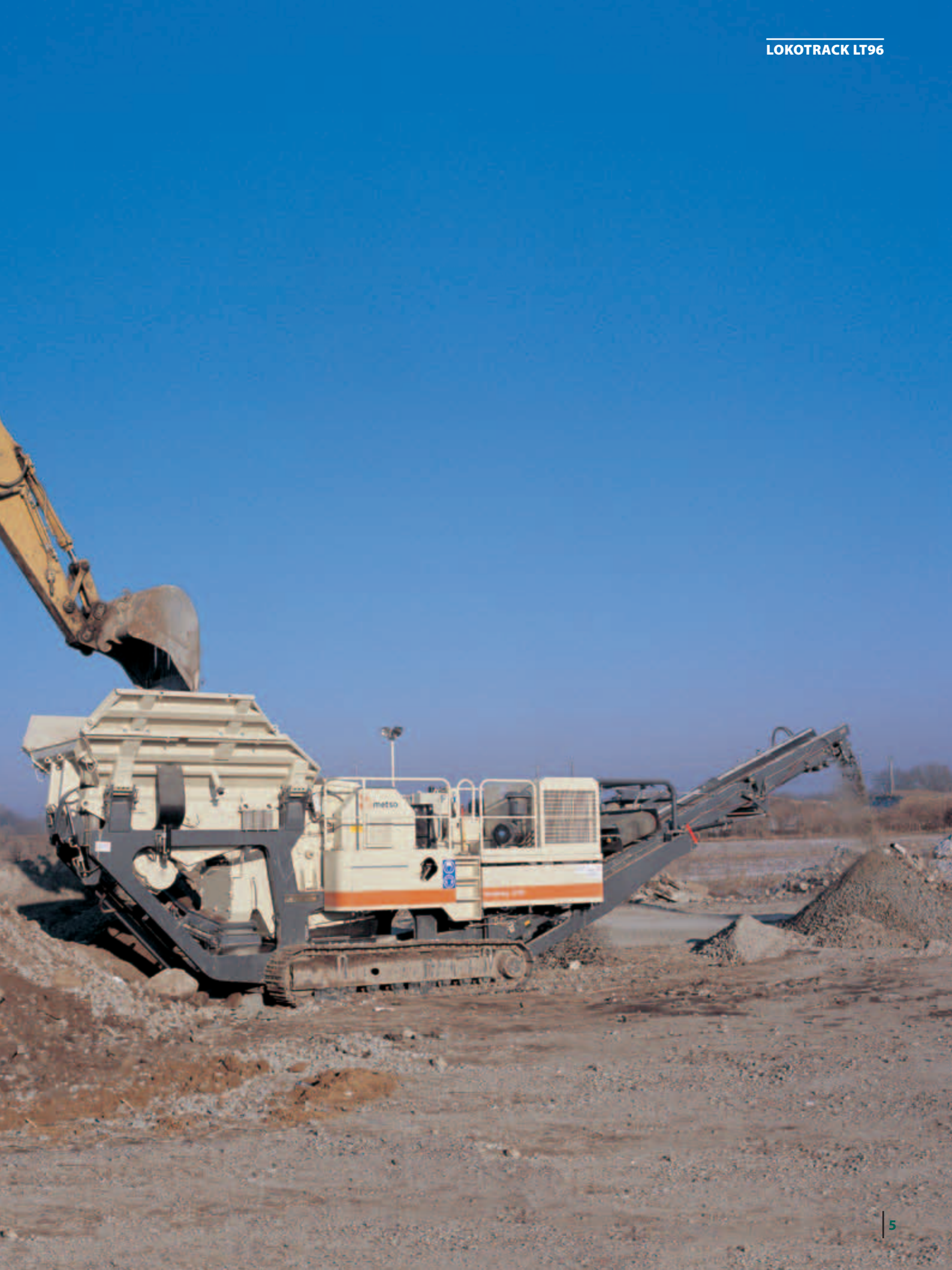
Another unique Lokotrack LT96 feature is the automatic locking mechanism for the feeder, cutting the time needed to prepare for transportation.
