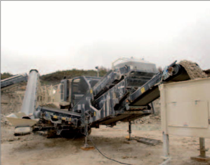
The screen of Lokotrack LT1213S can be opened easily for servicing and screen mesh change using the hydraulic system.
