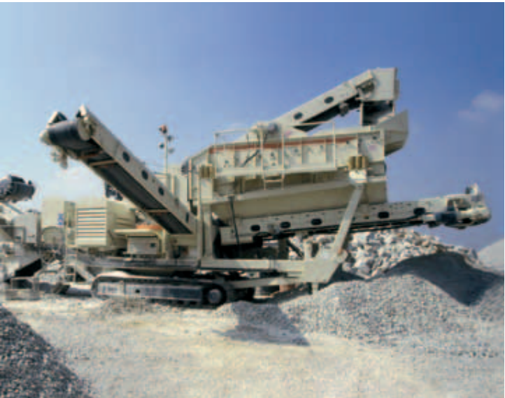
LT1100 can be transported easily between sites as a single unit on trailer.
