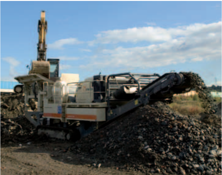
In addition to the standard conveyor, a longer, hydraulically folding conveyor is available.
