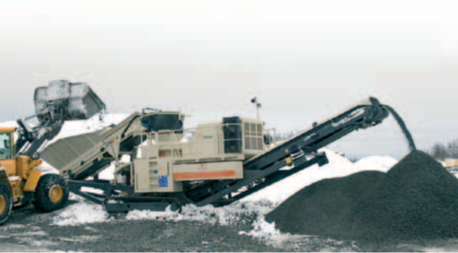
The IC600 intelligent control system ensures steady and constant crushing process.
