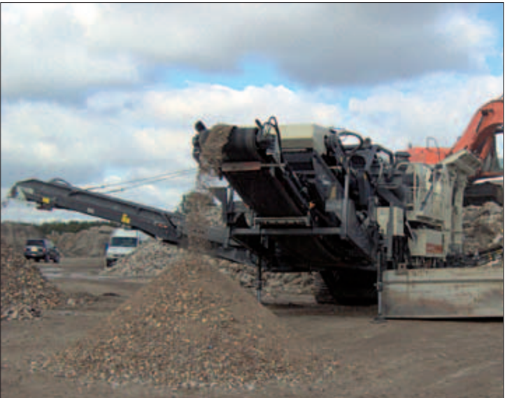
If needed, the screen module of LT116S can be detached quickly, and used with LT1213 and LT200HP models.
