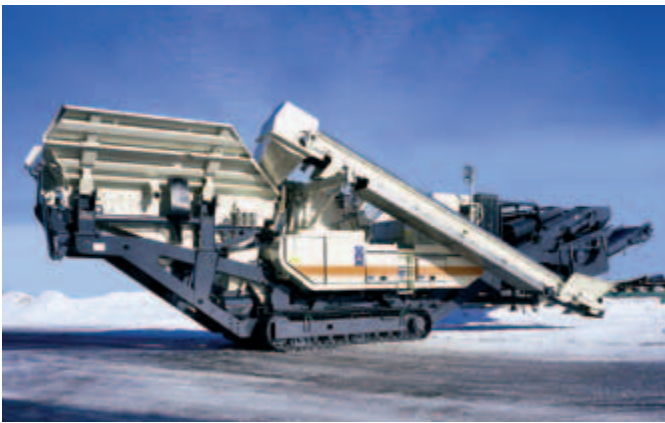
Lokotrack LT1110S impactor plant with a detachable screen.
