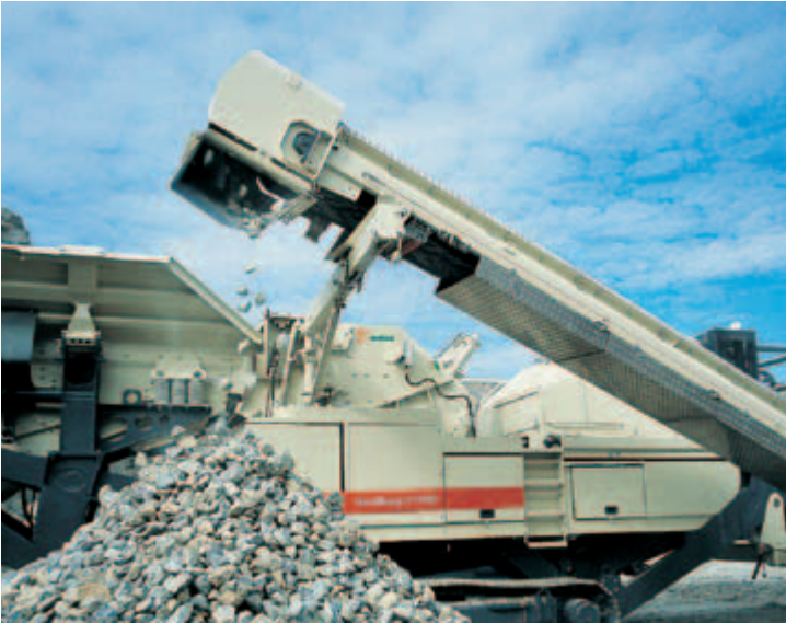
Two end products can be produced using an open circuit operation.
