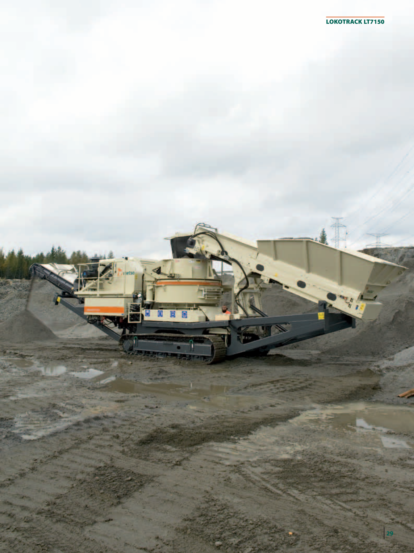
Thanks to the large feed hopper, LT7150 can be fed with conveyor, excavator or wheel loader.
