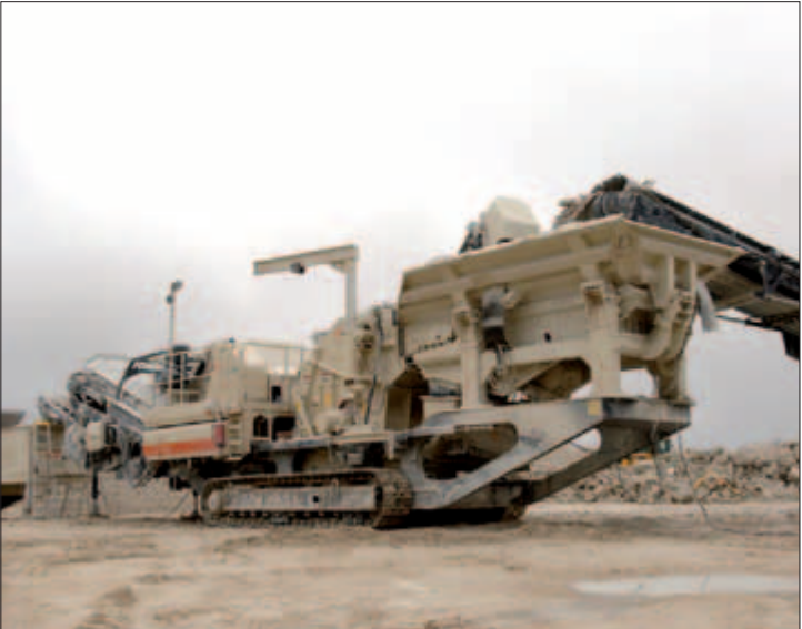
Lokotrack LT1213S crushing and screening limestone in Estonia.
