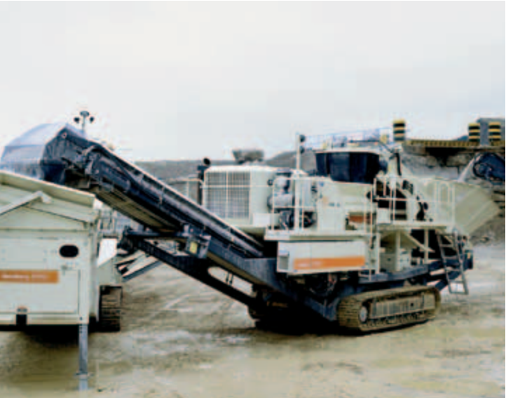
Lokotrack LT200HP can be easily operated with a primary impactor or jaw plant and with a mobile screen.
