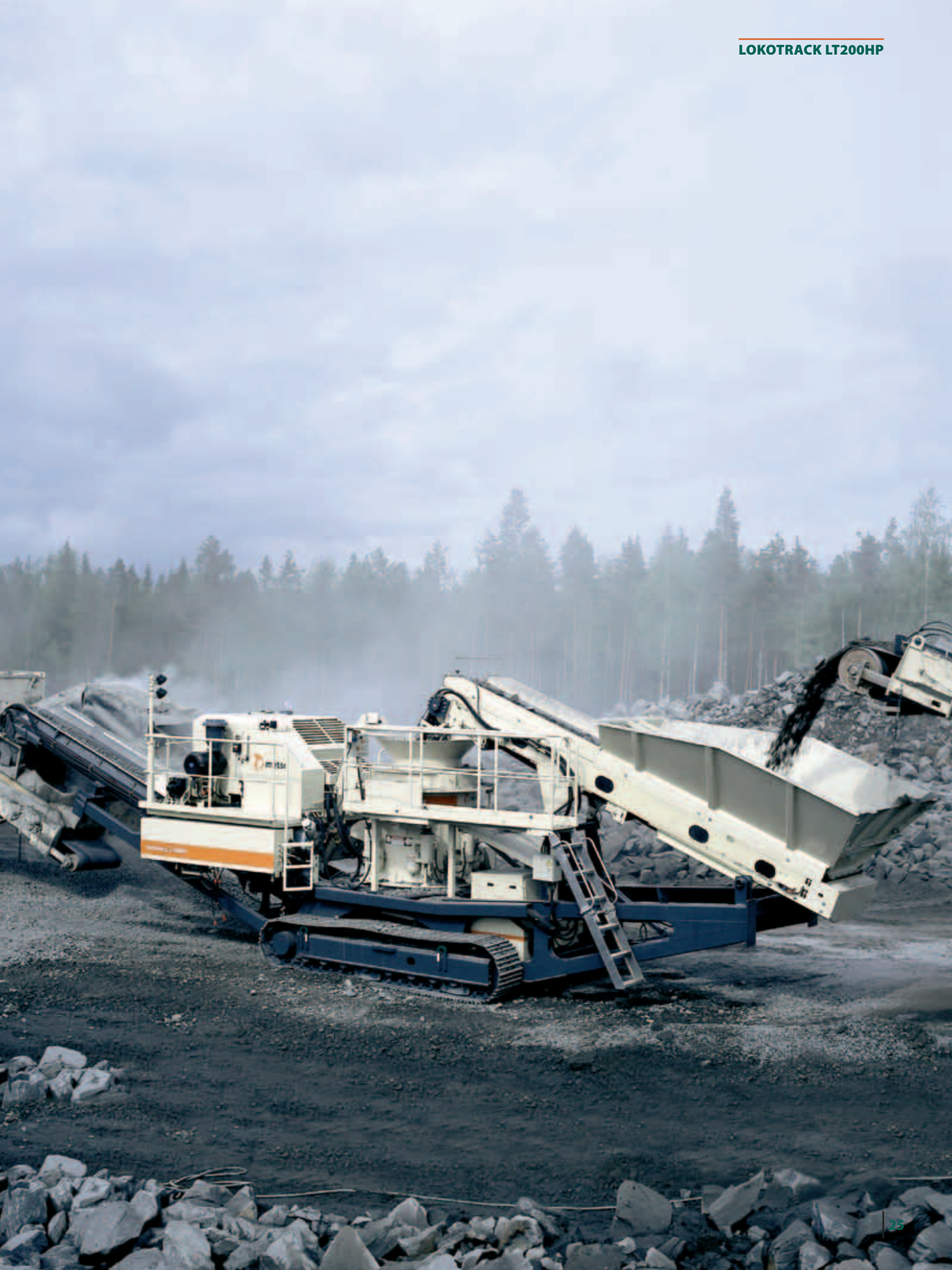
LT200HP is built around the proven and popular HP200 cone crusher.
