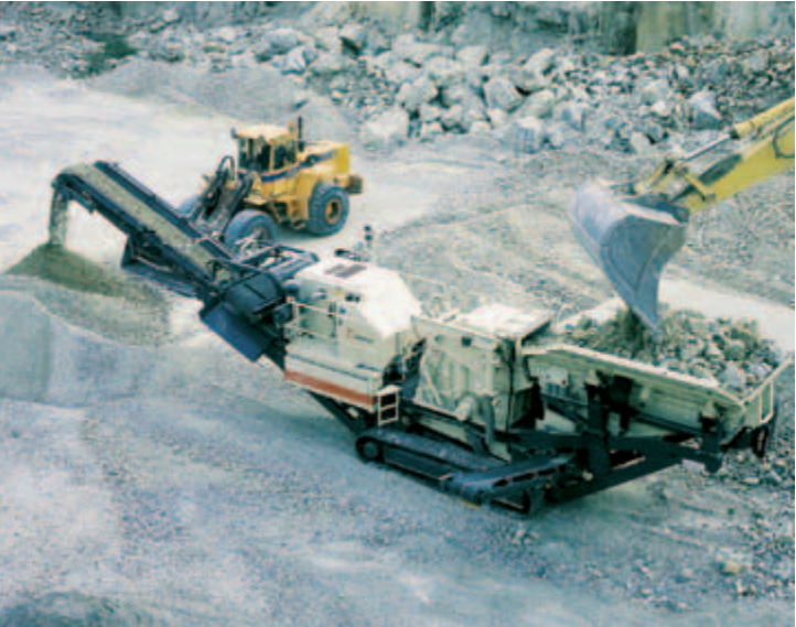
According to the application, Lokotrack LT1110 can be equipped with 5m 3 or 8m 3 sized feed hopper.
