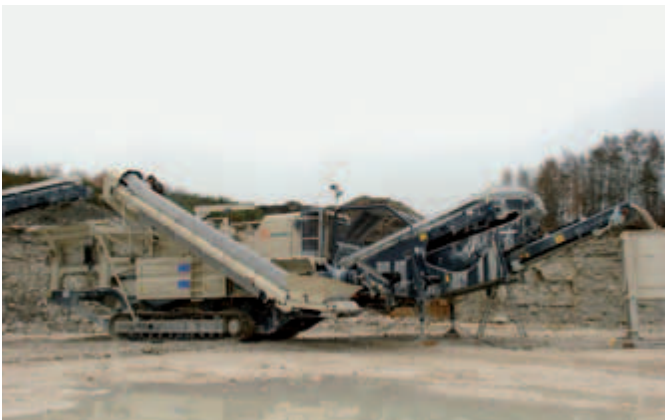
Lokotrack LT1213S impactor plant with a detachable screen.
