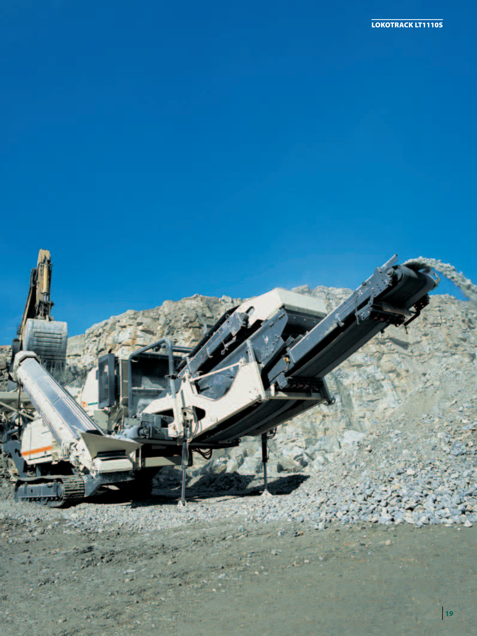
The two-directional rotation screen of Lokotrack LT1110S can be detached in minutes.
