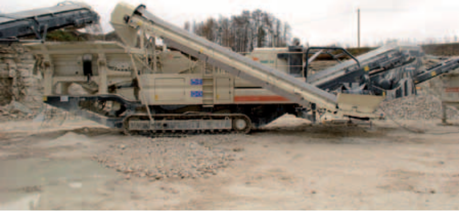
When used at closed circuit, the Lokotrack LT1213S produces one, exactly calibrated end product.
