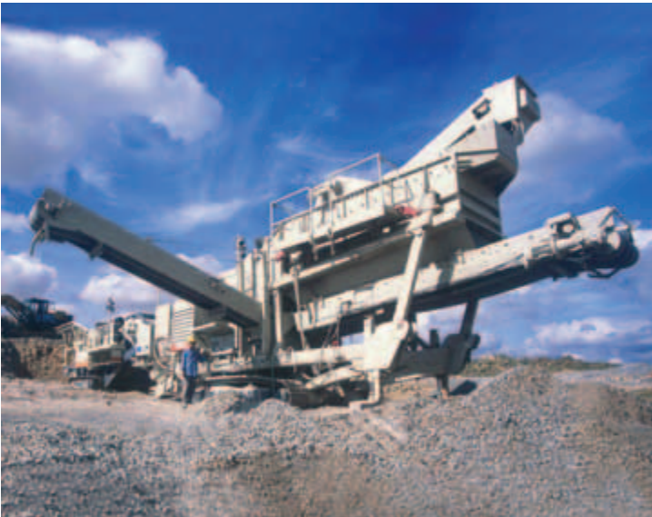
Nordberg GP11M or GP11F cone crushers can be selected to LT1100.
