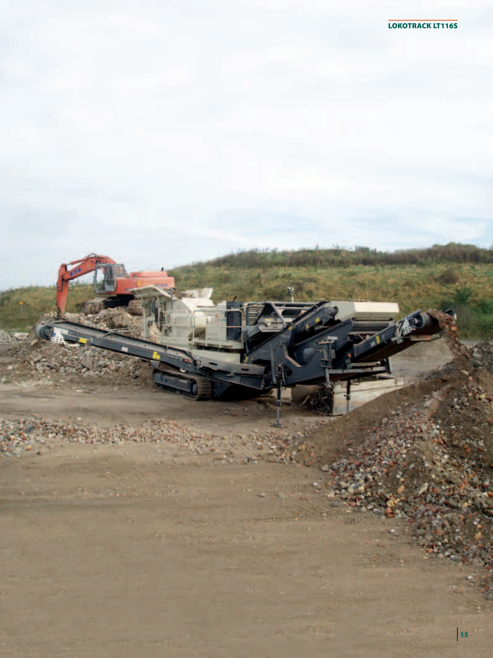
An optional magnetic separator can be selected for a recycle operation.
