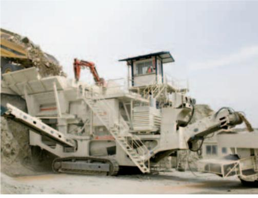
Lokotrack LT125 with an optional air conditioned control cabin.
