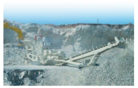
A mobile quarry application in Spain with a primary crushing plant LT140 and a TRLP12-20 conveyor.
