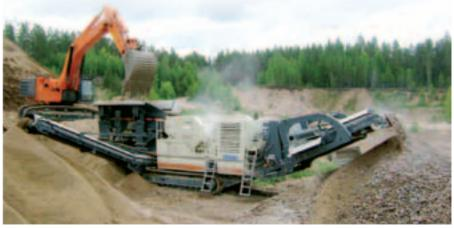
Road base materials crushed with LT3054 of natural gravel.
