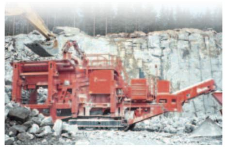
The "Split" model of Lokotrack LT125 is equipped with hydraulic legs for fast dismantling.
