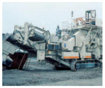
Recycle crushing with Lokotrack LT125 "Split" and LT300GPB in Germany.
