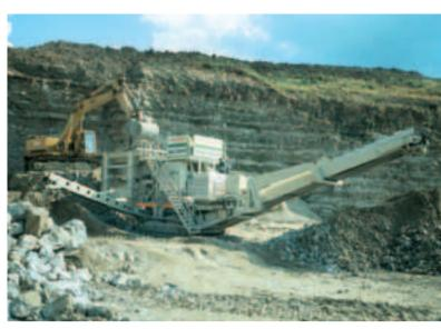
Primary crushing in the UK with Lokotrack LT125.
