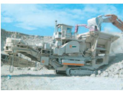
Mobile primary crushing for cement plant in the USA using LT140 + LL12.
