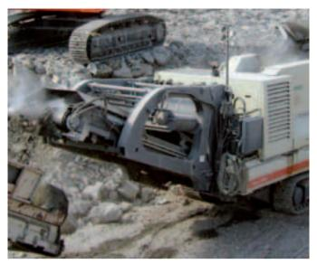
LT3054 at a two-stage crushing and screening process with a LT300GPB secondary cone plant.
