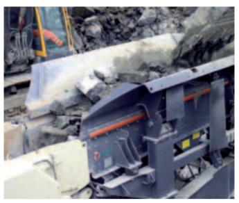
LT110 can be equipped with a high-capacity grizzly, a pan feeder/scalper or a roller grizzly.
