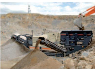
Fine materials can be removed before the crushing using a side conveyor.
