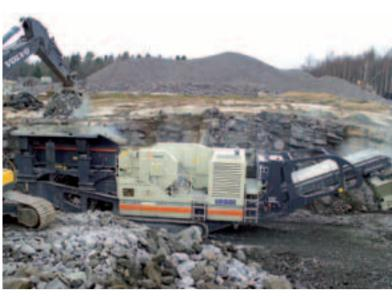
Primary crushing with Lokotrack LT110 in Sweden.
