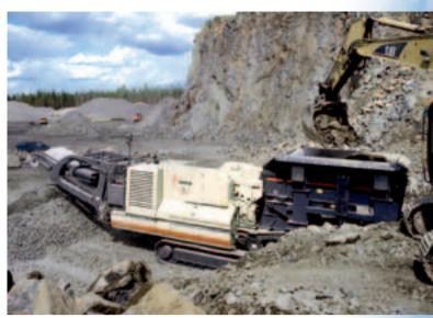
LT3054 features the one-button process start-up provided with the IC600 intelligent control system.
