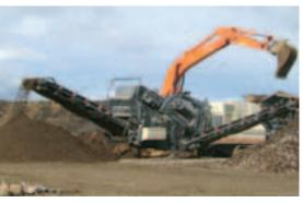
Lokotrack LT3054S, equipped with a screen module.
