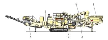
The track mounted Lokotrack LT300HP is the latest addition to the world renowned range of LT Series crushing plants. Equipped with HP300 cone crusher, LT300HP has a throughput of up to 550 mtph (660 stph).
